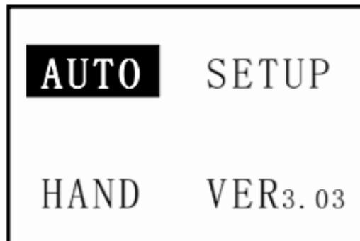
There are 7 screens in the automatic operation state, and the operation data of the power grid can be displayed cyclically by operating the up or down keys.
