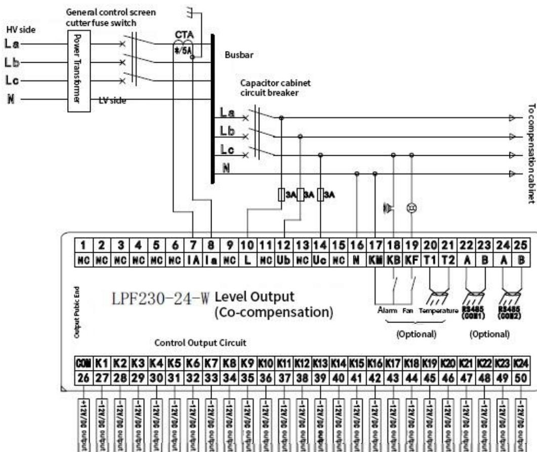
Note: 12 channels and 18 channels are only different in the number of control output circuits, and the other wiring is the same.
